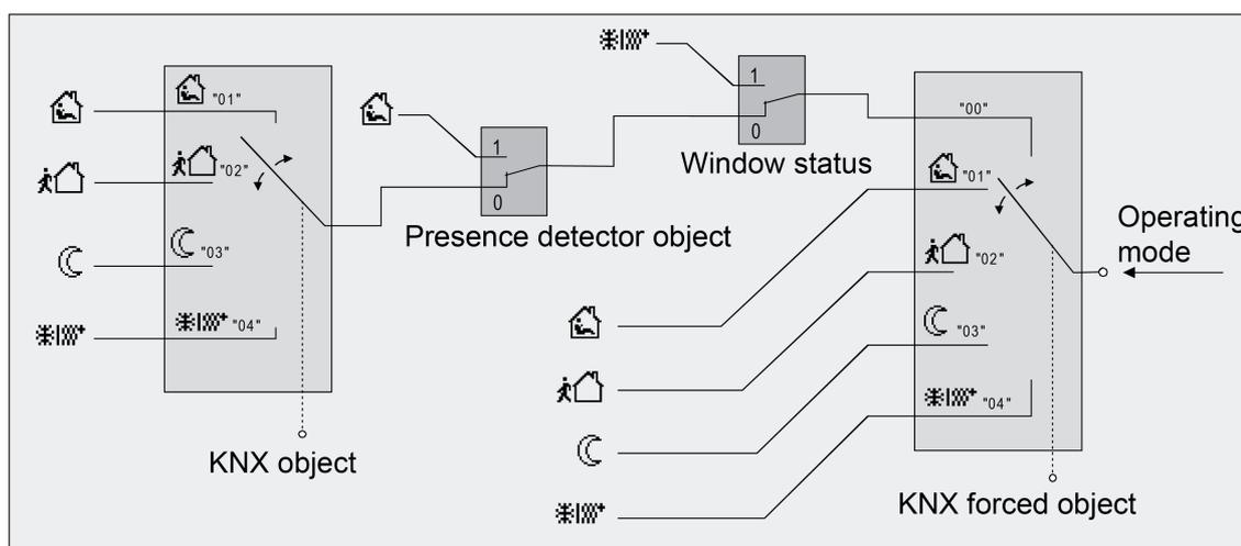
Figure 42: Operating mode switchover through KNX object with presence detector
