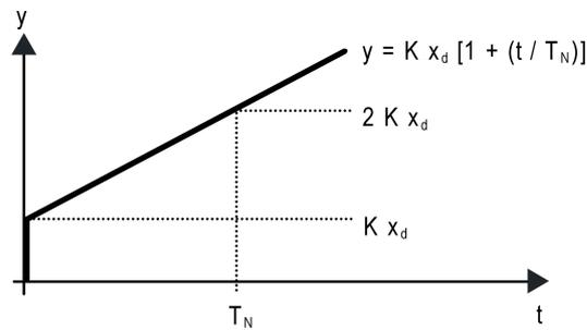
Figure 37: Function of the command value of a PI control
