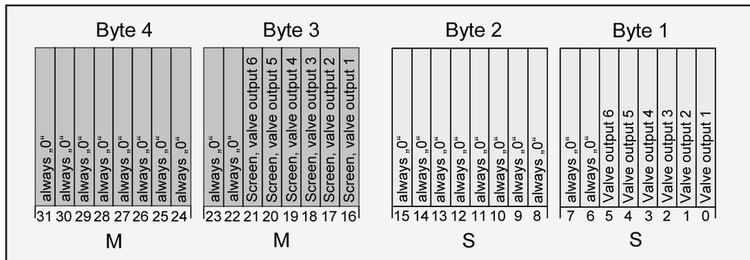
Figure 5: Object structure of the collective feedback
