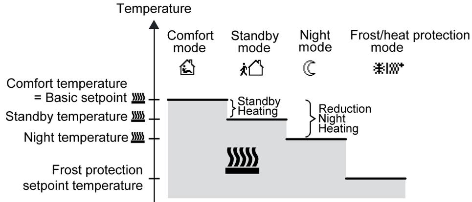
Figure 43: Setpoint temperatures in the operating mode "Heating"
