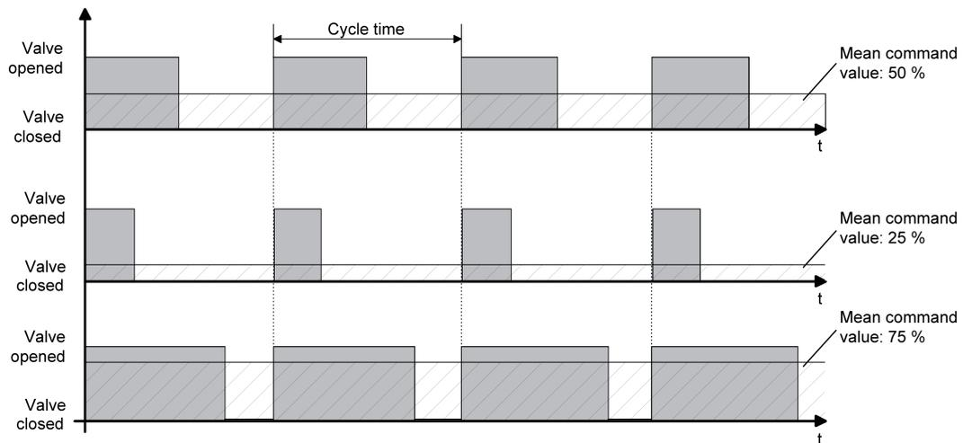
Figure 10: Resulting mean value through variable duty factor with pulse width modulation
