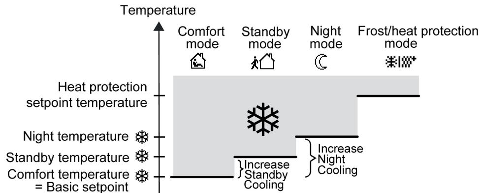
Figure 45: Setpoint temperatures in the operating mode "Cooling"
