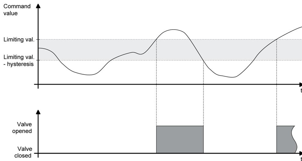
Figure 17: Example of command value evaluation with limiting value
