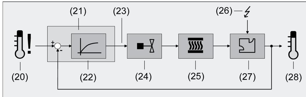
Figure 30: Controlled system of single-room temperature control
