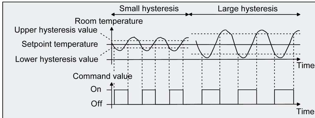
Figure 38: Effects of the hysteresis on the switching behaviour of the command value of 2-point feedback control
