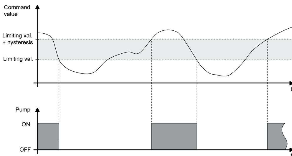
Figure 8: Pump control with sample command value characteristic
