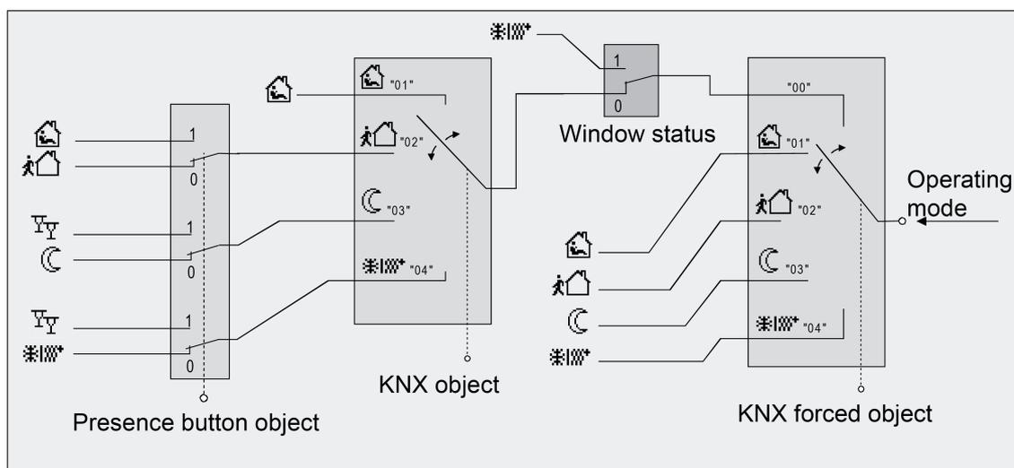
Figure 41: Operating mode switchover through KNX object with presence button
