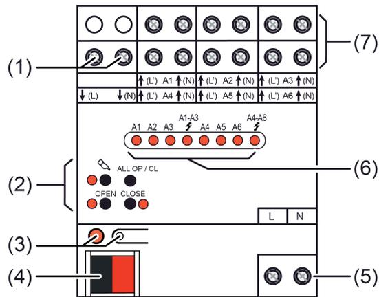
Figure 1: Device components
