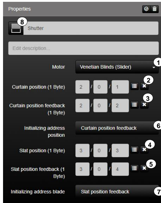
Figure 36: Parameters of the "Venetian Blinds (Slider)" function
