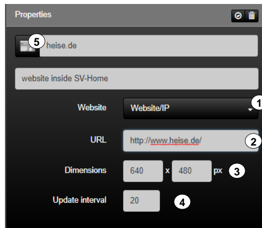
Figure 79: Parameters of the "Website" function
