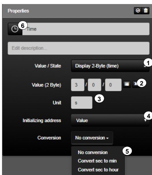
Figure 55: Parameters of the "Display 2-Byte (time)" function
