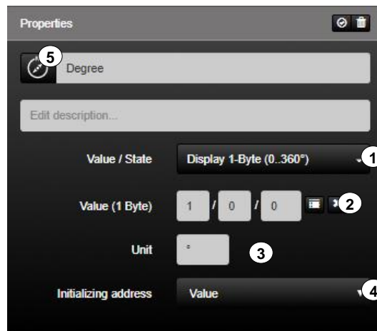
Figure 52: Parameters of the "Display 1-Byte (0...360°)" function
