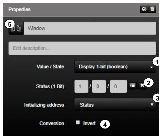
Figure 49: Parameters of the "Display 1-bit (boolean)" function
