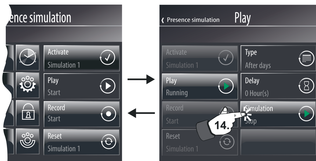
Figure 103: Example of a display page for starting and stopping a playback (right)
