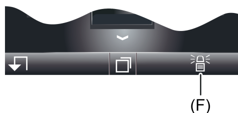
Figure 109: Symbol in the footer of the screen for displaying an alarm
