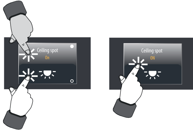
Figure 20: Example of sensor evaluation for direct operation (KNX function: Switching) left: rocker / right: button
