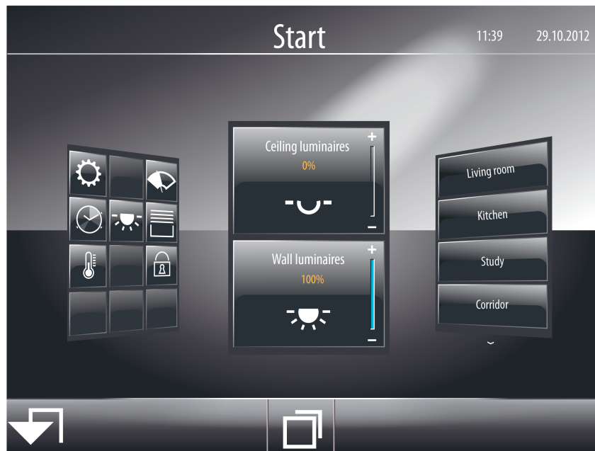
Figure 8: Example of a start page (2 operating and display functions with direct operation)
