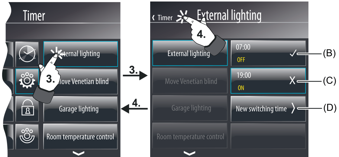
Figure 85: Example of a submenu for a timer switch channel with 2 switching times (right)
